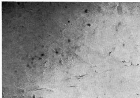
Fig. 1. Polished (100) face of potassium bromide, annealed at 370 °C for one hour. ( \times 200 ).
