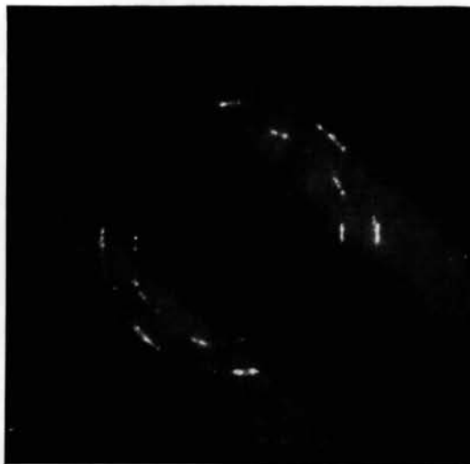
Fig. 6. Appearance of diffraction pattern with defocused objective lens.
